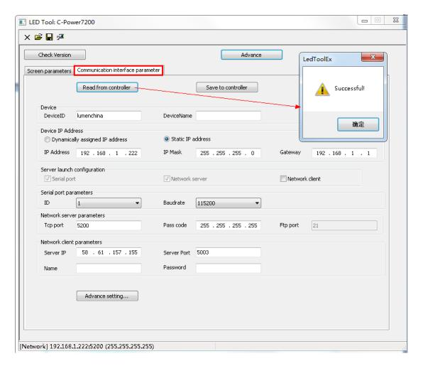
2. the communication interface parameter can be changed, click "advance" pass code is "26888", after resetting the data you want it to be, click "save to controller", when it successful, the controller will restart. As the following picture showed:
